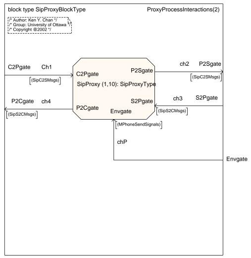
Figure 15: Block-Interaction Diagram of Proxy Type
