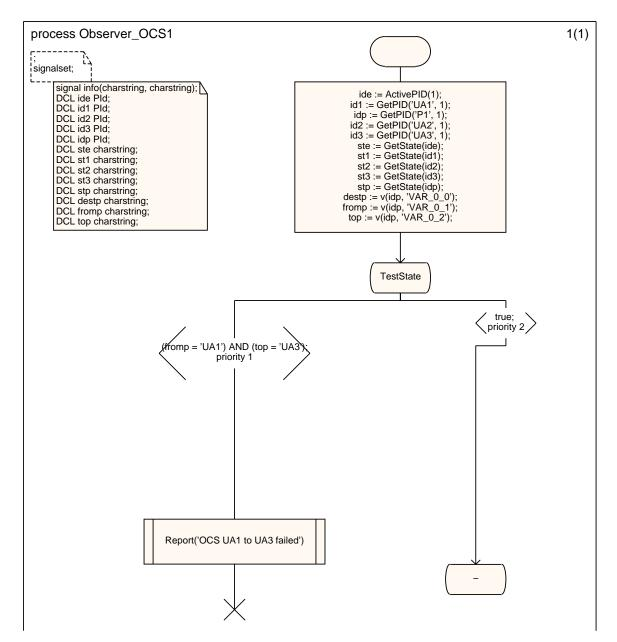
Figure 21: Sample Observer Process Assertion for OCS
