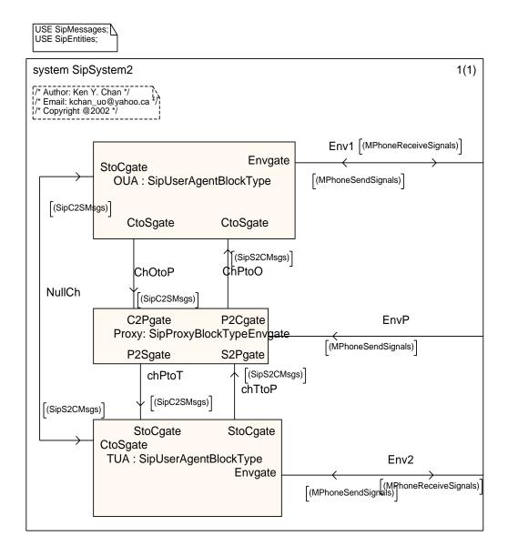
Figure 14: System Diagram of Proxy and User Agent
