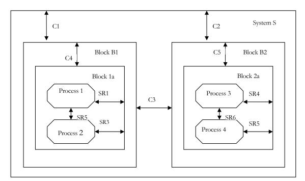
Figure 3: Basic SDL specification hierarchy
